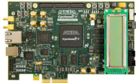
Figure: Intel/Altera Cyclone V SoC with FPGA
