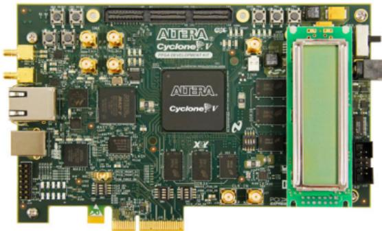
Figure: Intel/Altera Cyclone V SoC with FPGA
