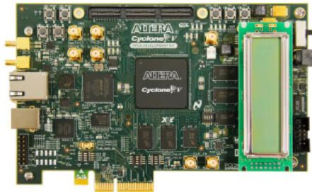
Figure: Intel/Altera Cyclone V SoC with FPGA
