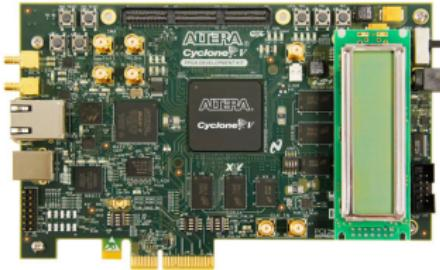
Figure: Intel/Altera Cyclone V SoC with FPGA
