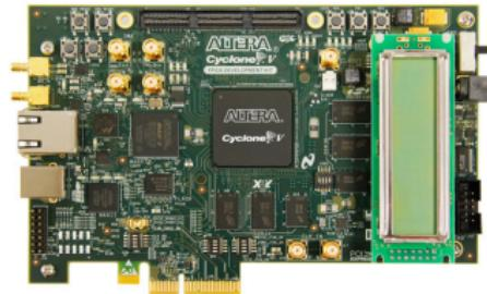
Figure: Intel/Altera Cyclone V SoC with FPGA
