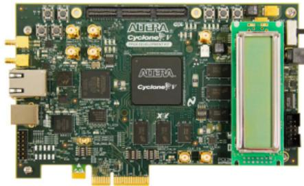
Figure: Intel/Altera Cyclone V SoC with FPGA
